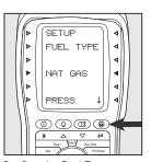
Confirm the Fuel Type. Scroll ▲ or ▼ to switch a different fuel type. Press ■ to select fuel type.
