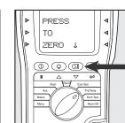
Press () "Pump" to ZERO (0) pressure sensor.
