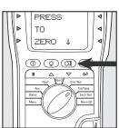
Press **Pump** to ZERO (0) pressure sensor.
