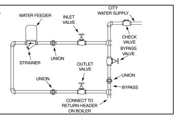
2. Water feeders are shipped from the factory equipped for a 2 gpm feed rate. A separate kit with instruction sheet and field installable orifices for 1 gpm and 4 gpm feed rates is included. If the alternate feed rates are required, refer to the instruction sheet provided with the kit for orifice replacement.
