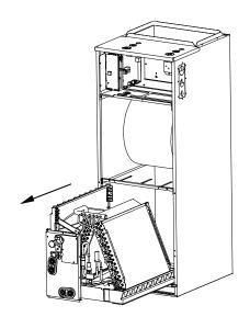
Fig. 20 — Remove and Rotate Drain Pan
