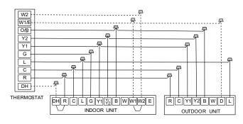
Fig. 65 —Wiring for 4H and 2C Thermostat
