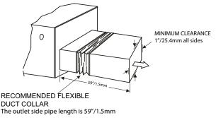
Fig. 28 — Flexible Duct Collar Connection
