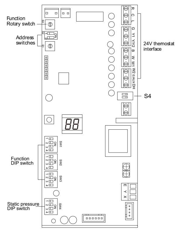
Fig. 54 — DIP Switches
