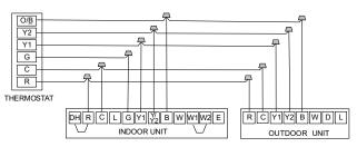
Fig. 69 —Wiring for 2H and 2C Thermostat
