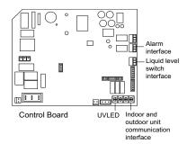
Fig. 57 — Optional Function Wiring
