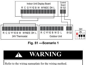
**DO NOT** connect 24V AC to S1-S2, as this will damage the system.
