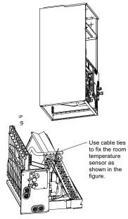
Fig. 24 — Assembled Evaporator
