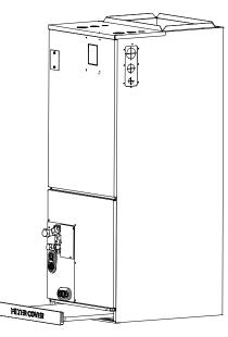
Fig. 15 —Remove the Filter
