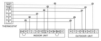
Fig. 70 — Wiring for 2H and 1C Thermostat
