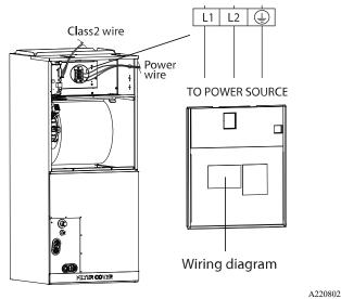
Fig. 49 —Indoor Unit Power Wiring
