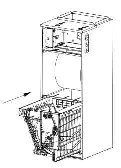
Fig. 22 — Reinstall Evaporator and Drain Pan
