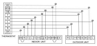
Fig. 66 — Wiring for 3H and 1C Thermostat
