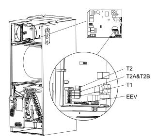
Fig. 18 —Unplug Temperature Sensors NOTE: T2A and T2B are only available for some models.
