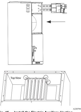
Fig. 45 — Install the Electric Auxiliary Heating Component
