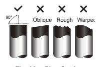
Fig. 32 — Pipe Cutting
