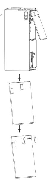
Fig. 43 — Remove the Upper Cover
