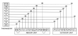
Fig. 68 —Wiring for 3H and 2C Thermostat
