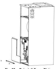
Fig. 25 —Reinstall Cover Plate
