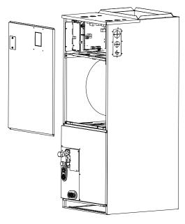
Fig. 16 — Remove Upper Cover Assembly
