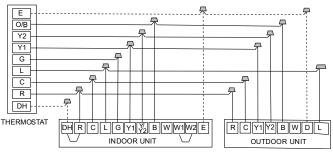
Fig. 67 — Wiring for 3H and 2C Thermostat
