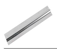
Heat transfer plates are used for Dry Below installations of 3/8",1/2" or 5/8" pex. Plates provide a direct transfer and heat distribution from Pex piping to the underside of a wooden subfloor. HeatTrak simplifies the installation by allowing the pipe to be snapped in place.
