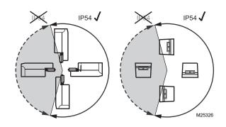
Fig. 8. Mounting for IP54.
