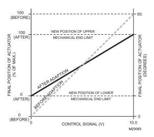
Fig. 5. Adaption (Function Selection Switch Set to 0...10 V).
