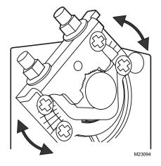
Fig. 6. Mechanical End Limits.
