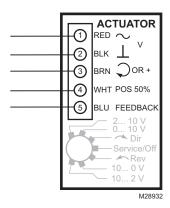
Fig. 14. MN7505W2001 Floating/Modulating/Two Position.
