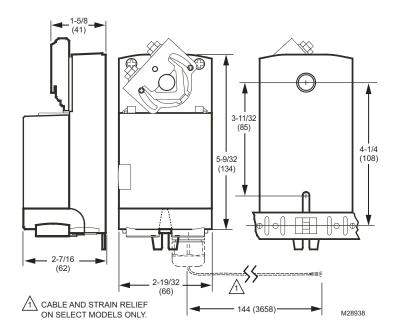
Fig. 15. Dimensions in Inches (mm).
