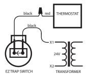
**Note:** Wiring diagram shown cuts power to thermostat when float switch operates to stop operation of the A/C unit. To inhibit mold growth during long absences, connect terminals into yellow cooling circuit so when float switch operates, condenser will switch off but fan will continue running.
