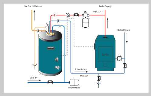
Alliance SL water heaters have a higher recovery rate than typical direct fired or electrically operated water heaters because they utilize the large output from the boiler as the heat source.
