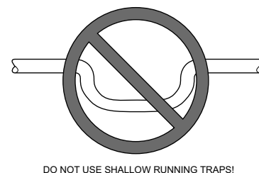
Fig. 12 – Insufficient Condensate Trap
