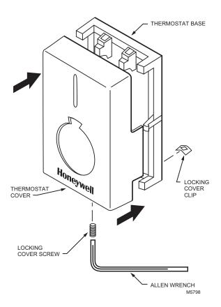
Fig. 8. Installing locking cover.
