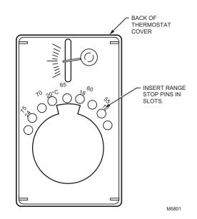
Fig. 9. Installing range stops.
