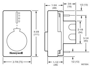
Fig. 1. T4398A,B dimensions in in. (mm).
