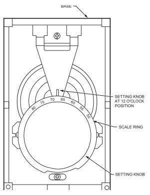
Fig. 7. Calibrating the thermostat.
