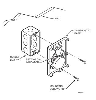
Fig. 4. Mounting thermostat to outlet box.
