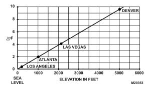
Fig. 5. T4398 altitude correction in (ft).
