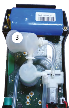
Sensor removed from white rubber cap
