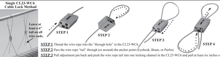
**STEP 3** Pull adjustment pin back and push the wire rope tail into one locking channel in the CL23-WC6 and pull at least six inches of the wire rope through. Failure to pull adjustment pin first may cause damage to serrated teeth and reduce holding capacity.
