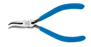
The 60-degree bent nose on these Midget Curved Chain-Nose pliers provide maximum work visibility in confined areas. This tool easily bends and forms fine wire. Polished inside jaws and radiused jaw edges prevent nicking wire while the curved handles provide greater tool control. Made of forged steel for maximum durability
