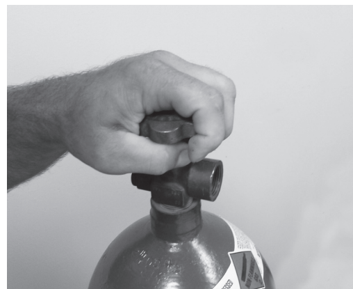
Figure 1. Opening Cylinder Valve
