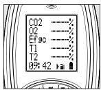
Flue 1 displays CO2, O2, Gross Efficiency, Flue temperature, Inlet temperature.
