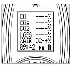
Flue 2 displays CO (ppm), Losses calculated, Excess air %. Make any adjustments needed for proper Combustion and wait for analyzer to display change in readings. (Repeat as necessary).
