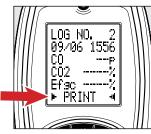
To print the LOG, Press ▲ and ▼ buttons until PRINT is selected between two arrow icons. Press ← to select to start printing.
