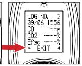
To EXIT, Press ▲ and ▼ buttons until EXIT is selected between two arrow icons. Press ← to EXIT screen.
