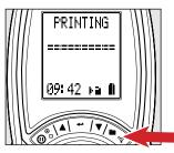
During testing, Press 훆 to start printing.
