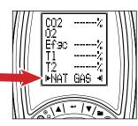
Press ▼ button until the Fuel Type displays on the Status Bar. Press and Hold ← until two arrow icons display.
