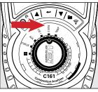
Rotate the function rotary dial to FLUE 2 for Flue Test Screen 2 parameters.
