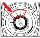
Rotate the dial to either AUX, FLUE 1, FLUE 2 or TEMP setting.
