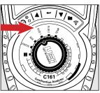
Rotate function rotary dial to FLUE 1 for Flue Test Screen 1 parameters.
