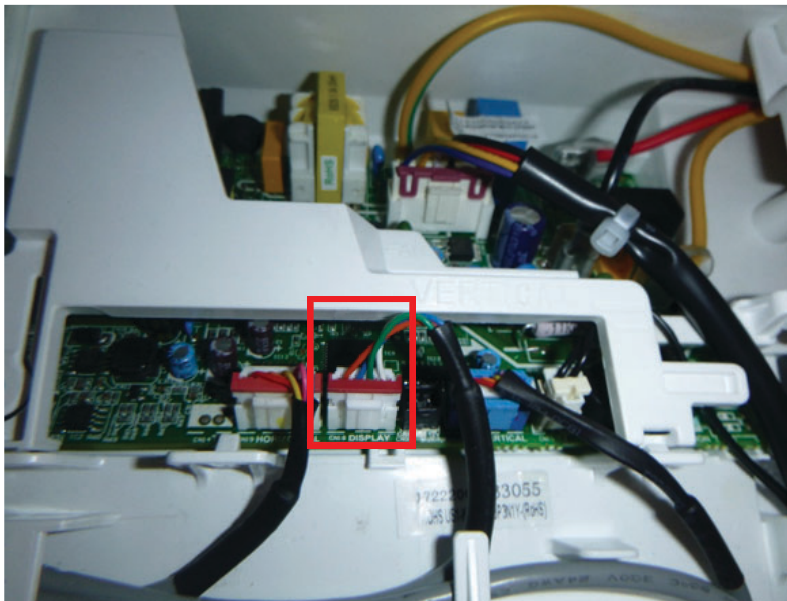
Fig. 14 — Remove the existing harness
