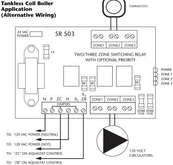
**Operation:** When the thermostat calls for heat, the appropriate circulator is energized and the isolated end switch  $(X_1 \text{ and } X_2)$  will start the boiler.
