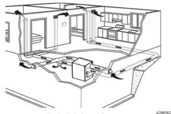
Fig. 5 - Fully Ducted System
