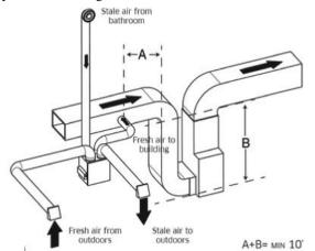
Fig. 6 - Exhaust Ducted System
