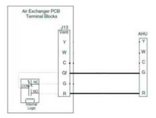
$\textbf{Fig. 20} - \textbf{Infinity} \\ \textbf{@/Evolution}^{TM} \ \textbf{Ventilator to AHU Wiring}^{A210005}$
