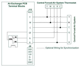
Fig. 18 – Wiring Options with Central Forced-Air System
