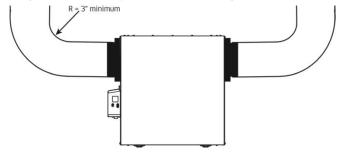
Fig. 13 - Correct Installation
