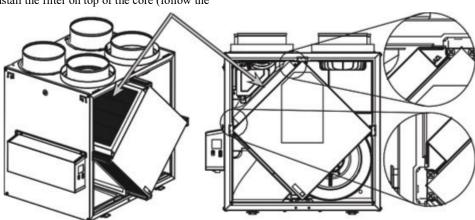
Fig. 28 – Optional MERV13 Filter or HEPA Membrane Filter
