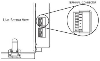
Use the terminal connector included to perform the electrical connection for optional main wall control. Check if all wires are correctly inserted in their corresponding holes in the terminal connector. Use screws to fix wires in the terminal connector. Once the wall control connections have been made, insert the terminal connector in the electrical compartment.
