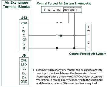
Fig. 16 - Wiring for Dry Contact Connection
