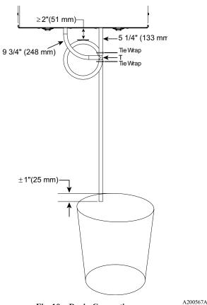
Fig. 10 – Drain Connection
