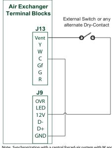
Note: Synchronization with a central forced-air system with W and Y is not available with this configuration.
