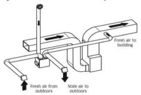
Fig. 7 – Exhaust Ducted System – Alternate
