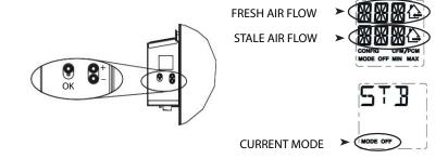
Fig. 22 - LCD Screen Buttons
