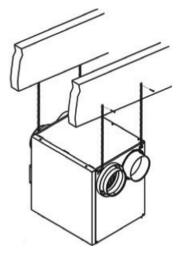
$Fig.\ 2-Suspended\ to\ Joist\ or\ Truss$
