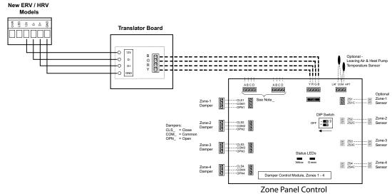
Fig. 19 - New Ventilator & NIM Connections
