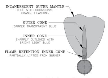
Figure 5: Main Burner Flame
