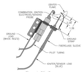
Figure 4: Pilot Burner
