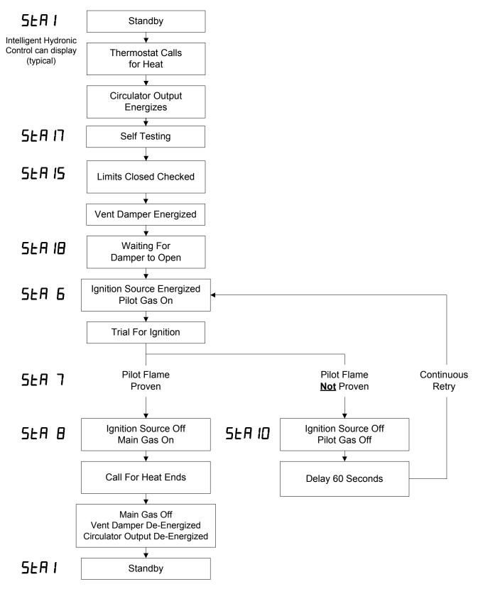
Figure 3: Sequence of Operation
