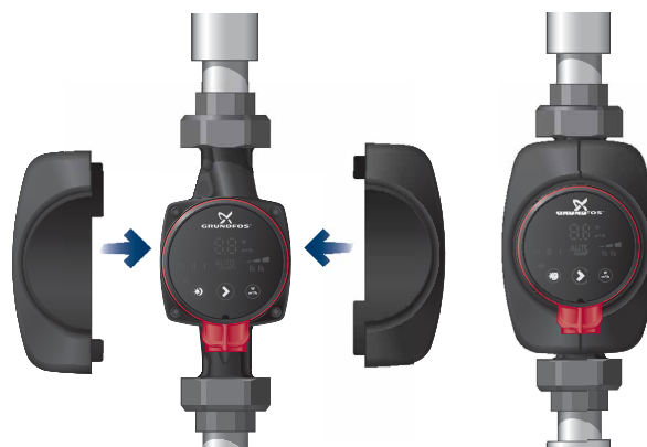
Fig. 10 Insulation of pump housing
