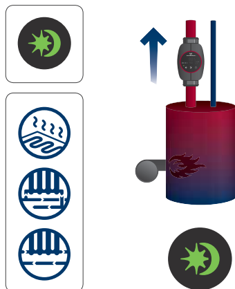
Fig. 23 Automatic night setback activated with the green light field on
