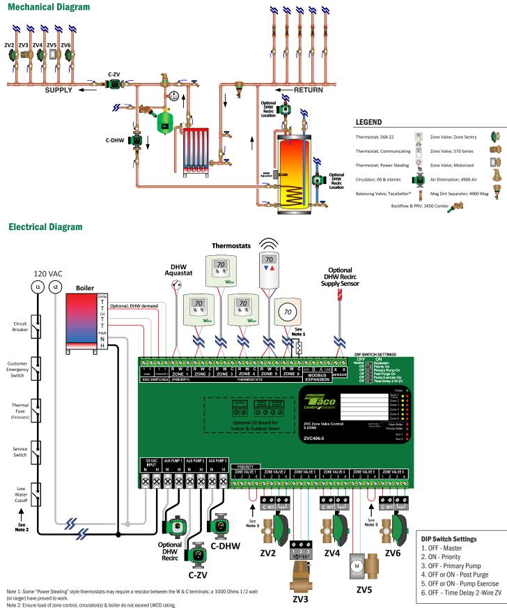
Note 3: If a 2 wire zone valve or no zone valve is used on individual zones then jumper 3 and 4 of that zone in order for the control outputs to activate
