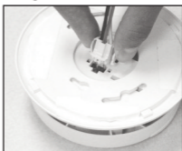
FIGURE 4 Installing AC Quick Connect
