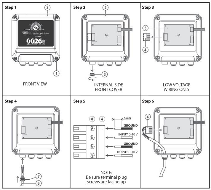
Figure 8 - External connection for 0-10V DC / PWM signal
