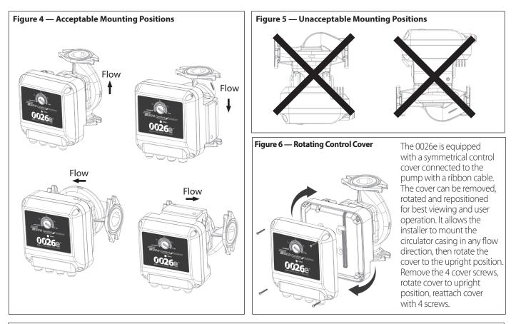
CAUTION: To reduce the possibility of noise transmission, be sure to add vibration dampeners to piping when mounting circulator to wall or floor joists.
