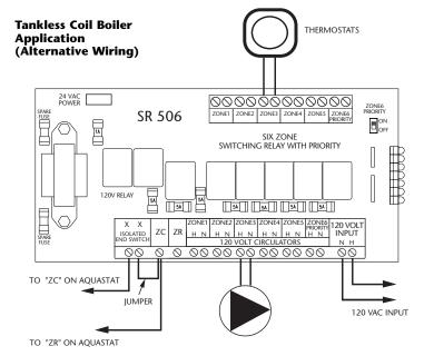
**Operation:** When any thermostat calls for heat, the appropriate circulator is energized and the isolated end switch (X and X) will start the boiler.
