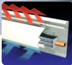
**Wall streakage eliminated.** Top panel and damper form a shield to keep dust from settling into baseboard interior, and to deflect heated air away from the wall, into the room. Back panel has no holes or slits to leak air behind the back of the baseboard causing wall streakage.
