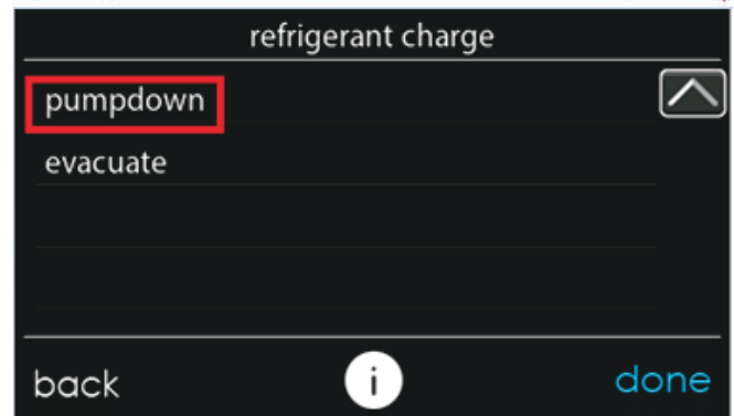
Fig. 24 – Pump Down and Evacuation Selection
