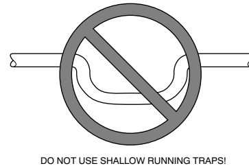
Fig. 13 – Insufficient Condensate Trap
