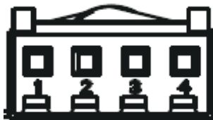
Fig. 15 – Sensor Wire Harness Pin Layout
