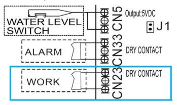
Fig. 59 —WORK Terminal Port CN23
