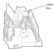
Fig. 26 — Use cable ties to fix the room temperature sensor
