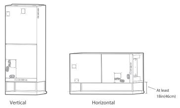
Fig. 10 — Vertical or Horizontal Installation
