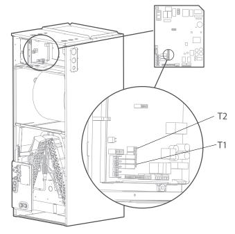
Fig. 19 — Unplug Temperature Sensors
