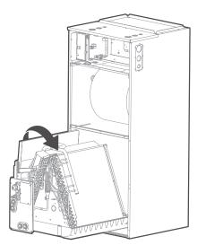
Fig. 21 — Remove the evaporator and drain pan
