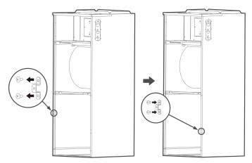
Fig. 22 — Adjust the mounting parts position
