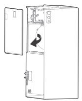
Fig. 14 — Remove the upper cover assembly
