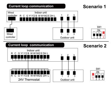
Fig. 52 —Connection Methods for 18K-36K Residential Units
