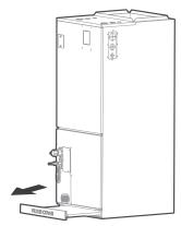
Fig. 13 — Remove the filter door
