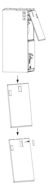
Fig. 43 — Remove the Upper Cover
