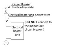
Fig. 51 —Wiring Connection of Electric Heater (optional)
