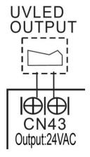
Fig. 62 —UV LED Terminal Port CN43
