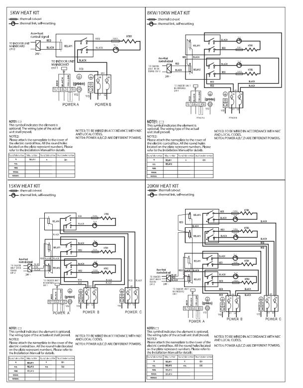
Fig. 64 — Electric Auxiliary Heating Wiring Diagram
