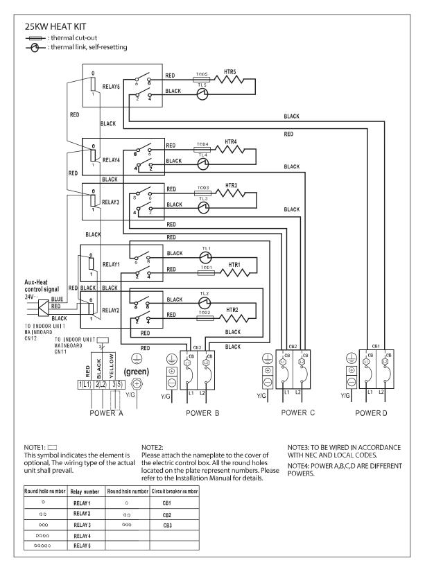
Fig. 65 —Electric Auxiliary Heating Wiring Diagram
