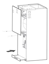
Fig. 28 — Reassemble the upper cover and filter
