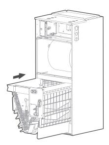
Fig. 23 — Reinstall the evaporator and drain pan
