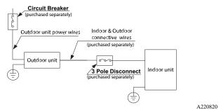
Fig. 50 —Wiring Connection of Indoor Unit
