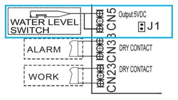
Fig. 61 —WATER LEVEL Terminal Port CN5
