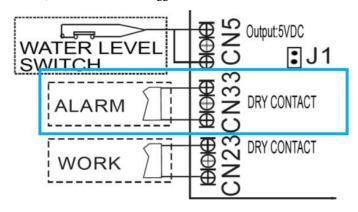
Fig. 60 —ALARM Terminal Port CN33
