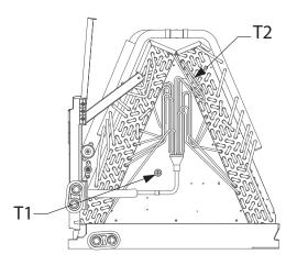
Fig. 18 — Temperature sensor position
