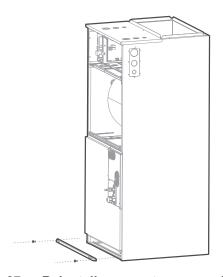
Fig. 27 — Reinstall evaporator cover plate
