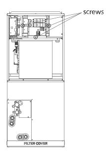
Fig. 46 — Tighten the Screws
