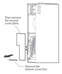
Fig. 15 —Remove the evaporator cover plate
