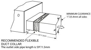
Fig. 29 — Flexible Duct Collar Connection
