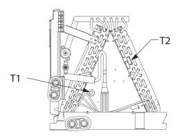
Fig. 16 — Temperature sensor position
