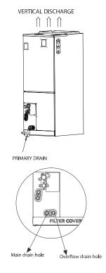
Fig. 30 —Vertical Discharge
