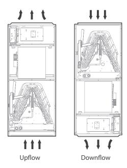
Fig. 11 — Vertical Airflow
