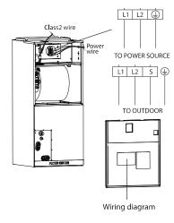
Fig. 49 —Control Box and Wiring Diagram
