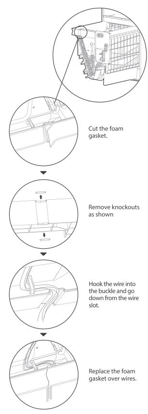
Fig. 24 — Reinstall T1, T2 sensor plug and tie up the sensor wires
