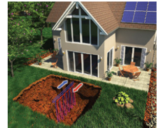
Vertical Ground Loop System
