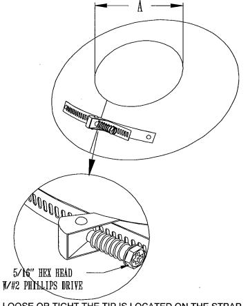
ØA & ØB CAN VARY +/- 1/2" DEPENDING UPON HOW LOOSE OR TIGHT THE TIP IS LOCATED ON THE STRAP
