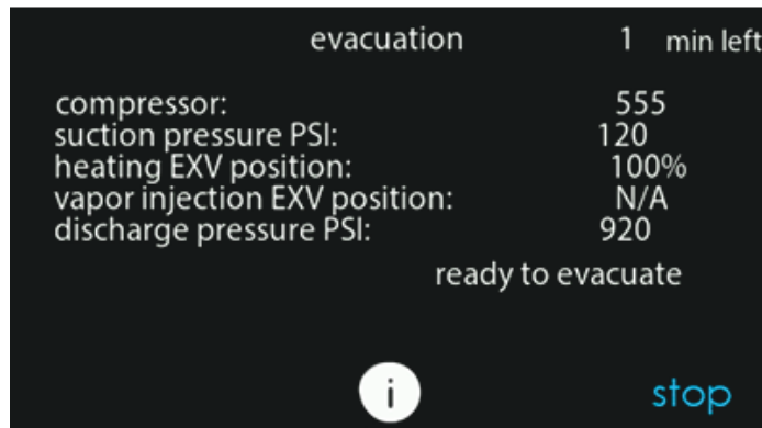
Fig. 44 – Evacuation Status Screen
