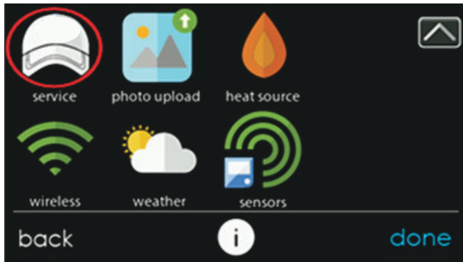
Fig. 38 – Entering Installation and Service Menu A200029
