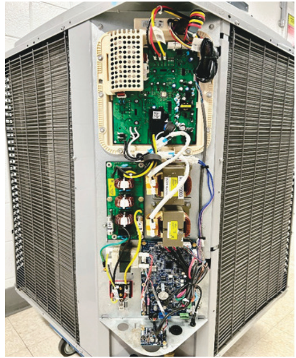
Fig. 21 – 4/5T Control Box Note: 4T VFD similar, not exact. 5T reactors have additional chokes and are routed differently to meet FCC requirements
