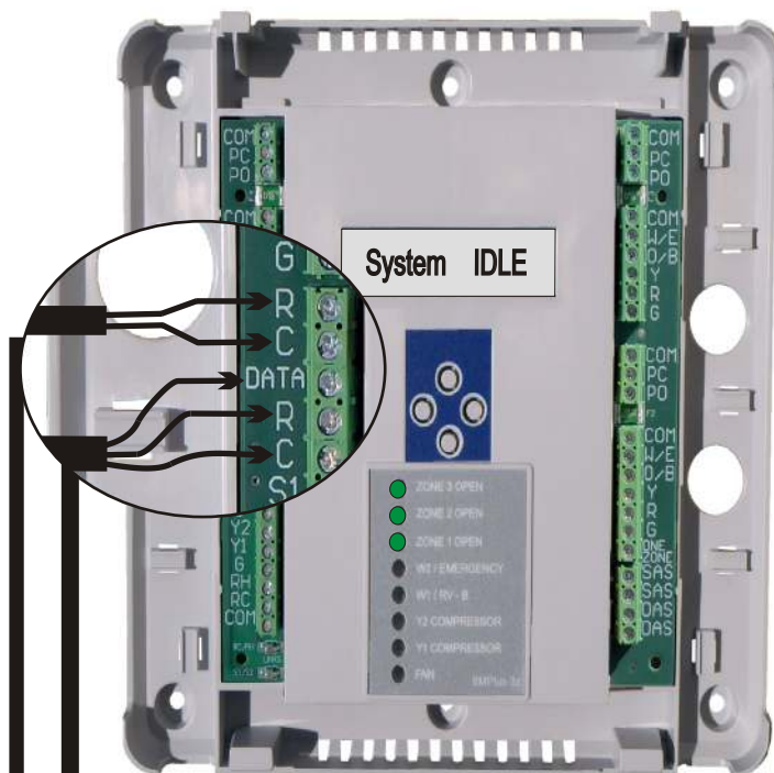
BMPlus-3z with 3 WiFi Tstats = 16va power load
