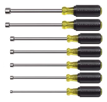
The Klein Tools 7-Piece Magnetic Nut Driver Set features nut drivers with internal flanges to provide a solid, twist-resistant shaft anchor. The nut drivers are made with chrome-plated, hollow shafts to help prevent corrosion. The donut-shaped magnetic tips easily hold fasteners in place for convenient use. The drivers are constructed with Cushion-Grip handles to provide greater torque and comfortable use.
