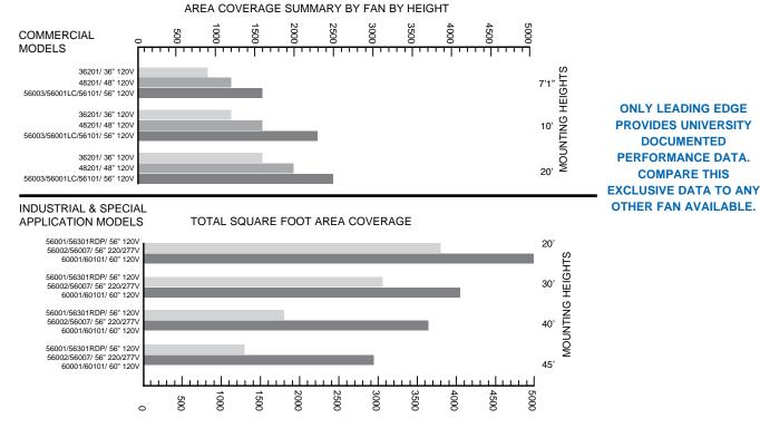
APPLICATIONS: Educational facilities, offices, retail stores, restaurants or any other low ceiling application where larger blade diameters span creates maximum air velocity and area coverage at lower RPM's.
