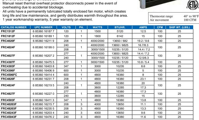
\*Factory wired for higher wattage, field convertible to half wattage. Standard finish: Statuary bronze. For Northern White finish, please add NW suffix to catalog number when placing an order.
