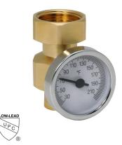
Caleffi 521 and 5231 series mixing valves are available with optional outlet temperature gauge, or field installed with point of distribution low-lead brass mixed temperature gauge adapter (above) replacing the existing threaded union outlet nut and tailpiece. Removable 2" gauge fits into temperature well.
