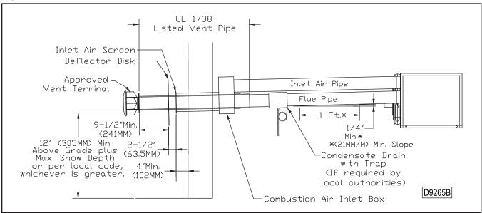
▲ WARNING Never use pipe other than 4 inch diameter. Never use PVC, ABS or any other nonmetallic pipe for venting! To do so may result in serious damage to the unit and or severe personal injury or death!
