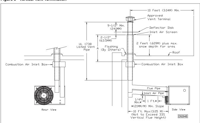
**Figure 6 - Vertical Vent Termination**
