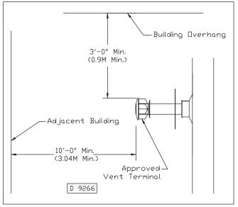
Figure 5 - Horizontal Vent Termination
