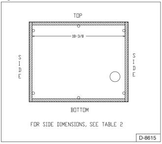
**Figure 4 - Horizontal Vent Termination Location**
