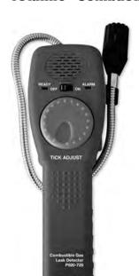
Easily operate the P920-720B with one hand while detecting the presence of combustible gases including natural gas, methane, propane (LPG), gasoline, diesel, and kerosene Pinpoint leak sources with its audible and visual indicators. An adjustable "tic" rate helps eliminate background gas concentration in contaminated environments.
