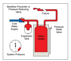
Plumbing codes and water heater manufacturers' warranties often require a water heater expansion tank. See the sizing charts below and select a Therm-X-Trol<sup>®</sup> model to protect your system.
