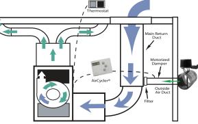
is recommended to install with the motor at the 12 o'clock position it mounted horizontally. Air may flow through in either direction, although it is recommended to install with the crimped end as the outlet of the damper. Use care to avoid distorting the damper housing, and provide adequate support.
