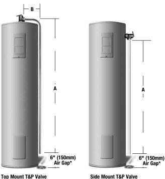
\* Drain tube must be trimmed to 6" (150mm) above drain so that any relief discharge will be visible.
