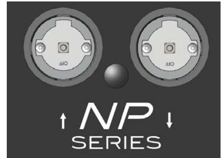
Figure 7: Valve positions for flushing with flush cart. OFF is in 6 o'clock position.
