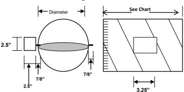
All dimensions are nominal. Dampers 10" diameter and less are 9.75" in length. Dampers 12" and over are .250" shorter in length than the diameter.
