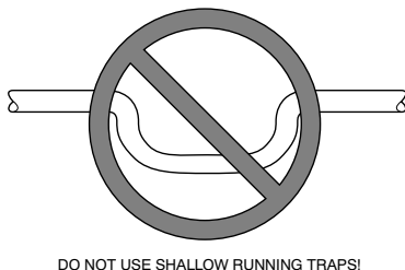
Fig. 5 – Insufficient Condensate Trap
