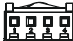
Fig. 7 – Sensor Wire Harness Pin Layout
