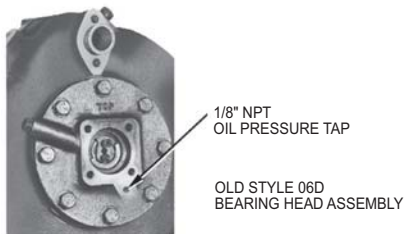
Fig. 11 — 06D 6-Cylinder Compressor (25, 28, 37, and 41 Cfm) Connection Points
